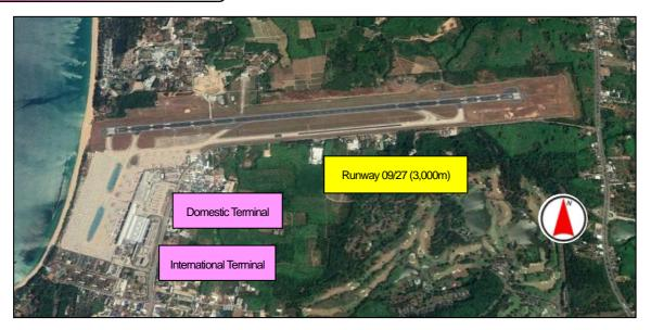
The airport is at an elevation of 25m above mean sea level. It has one runway designated 09/27 with an asphalt concrete surface measuring 3,000m x 45m.
